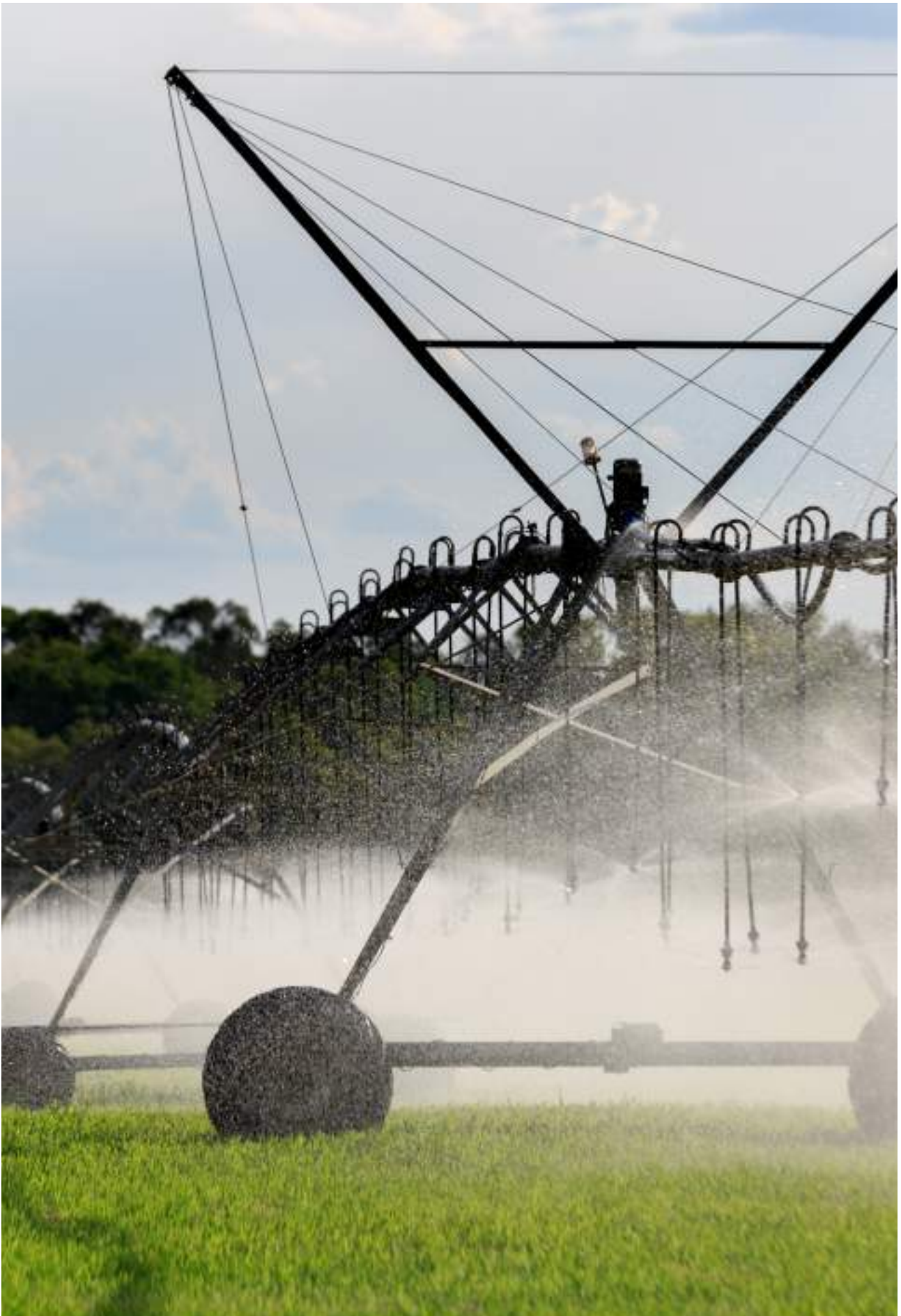
Lateral Move Irrigation System
